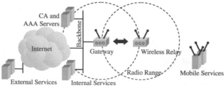
Fig. 4. The basic infrastructure provided by the TSP includes the wireless mesh network, CA and AAA servers and other internal and external services.
